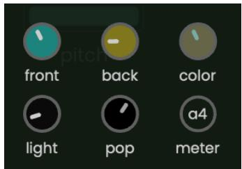
Controls for the appearance of SweetEQ and style of the spectrogram lines. Click and drag on a knob to change its value. Control the primary (**FRONT**) and secondary (**BACK**) colors, how much **COLOR** is in the background and faders, how **LIGHT** the background is, how much the faders **POP**, and the **METER** appearance. The numbers in the meter mode correlate to the thickness of the bars. The letters describe the style:
